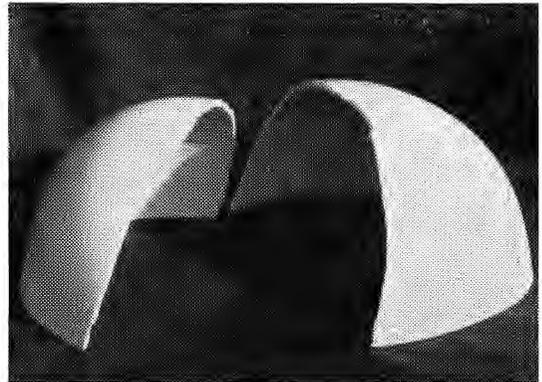
**Fig. 11** Seven point half months exposd ABS (2.3kg)
