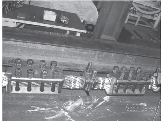
Photo.3 Wire grip loading test using M- type grips.
