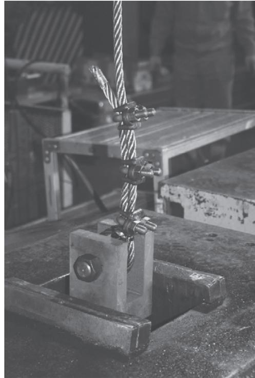
Photo.1 Wire grip loading test for small diameter ropes.
