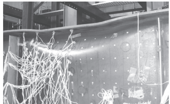
Photo.3 Destruction situation (Excessive deformation). 無補強部の最大耐力以降の過大変形状況
