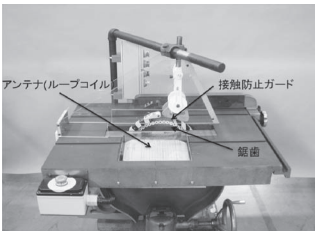
Photo 1 The appearance of safety system for circular saw developed in this research. 丸のこ盤の安全システムの外観
