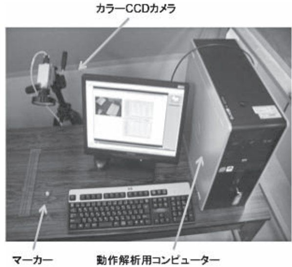
Photo 2 The appearance of experimental equipment for measuring the speed of human hands. 手の速度の計測実験装置の外観
