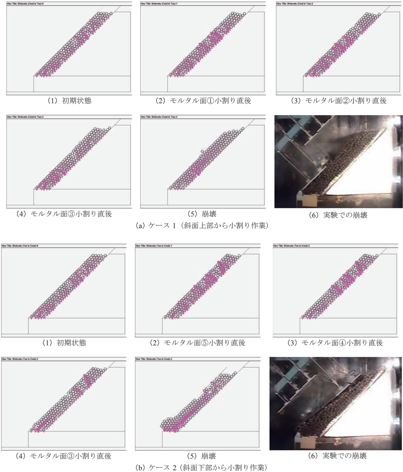
Fig. 8 Analytical results simulated by centrifuge model test.
