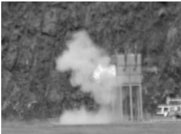
Photo 9 Aspect of explosion venting in 1m 3 vessel(still photographed) 1m 3 容器における爆発放散の様子
