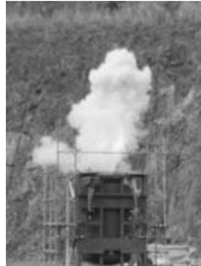
Photo 13 Aspect of explosion venting in 6 m 3 vessel ( still photographed at observation point 2).
