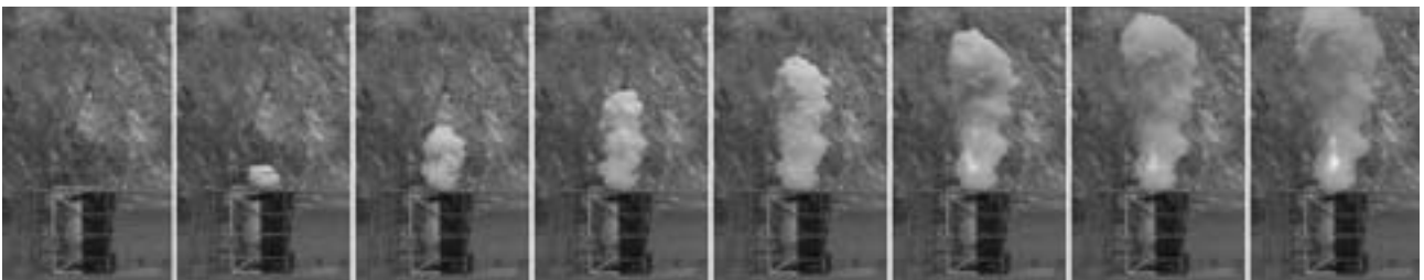
Photo 14 Sequence of explosion venting in 6 m 3 vessel ( photographed by camcorder) (picture is every 33 ms from left to right.)
