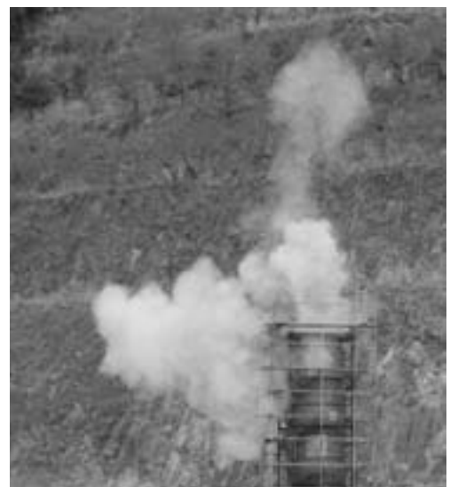
Photo 16 Aspect of explosion venting in 20 m 3 vessel (still photographed at observation point 2).
