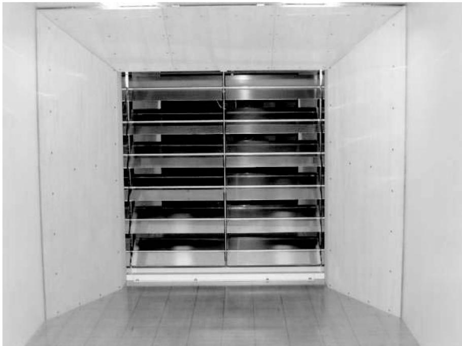
Photo3 Gust generation system set in the first measurement area.
