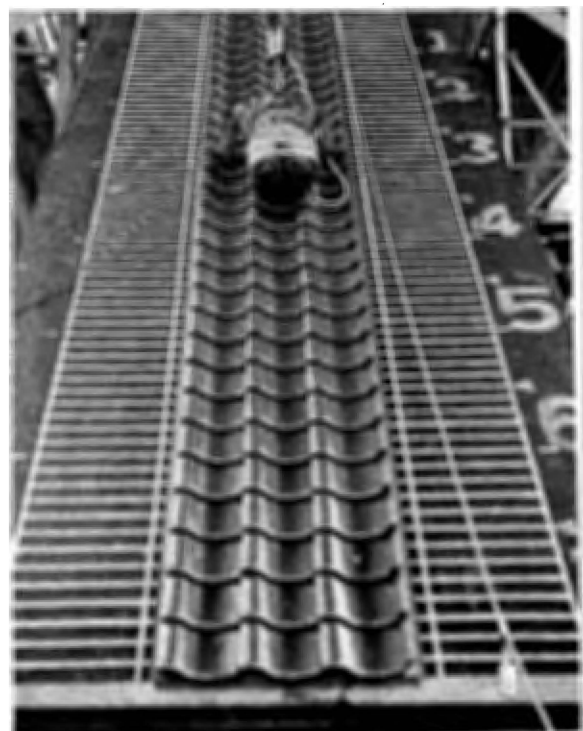
Photo. 2 Mimic roof laid with tiles 瓦葺模擬屋根
