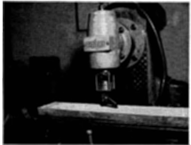
Fig. 3-2 Test for anti-kickback finger 反発防止爪の試験
