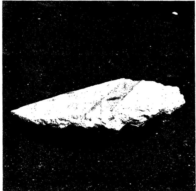
Photo 5.3 Concrete fractured in shape of a circular cone
