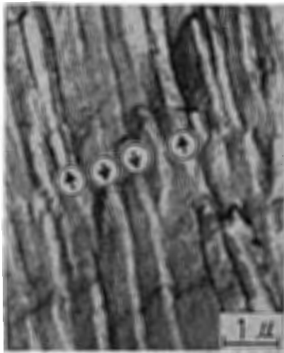
Fig.3 Striations observed between lamellar cementite (indicated by arrows) in the material annealed at 850°C 850°C 焼なまし材の層状セメンタイト(矢印)の間に見られるストライエーション \Delta K=76.9 \text{ kgmm}^{-3/2} , R=0 , dl/dn=0.089 \mu/c
