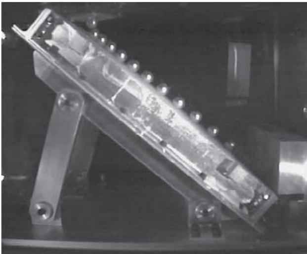
Photo 8 Typical example of simulated trajectory of falling aluminum sphere (RF-01-7).
