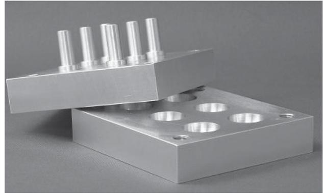
Photo 5 Mixture spheres making mold.
