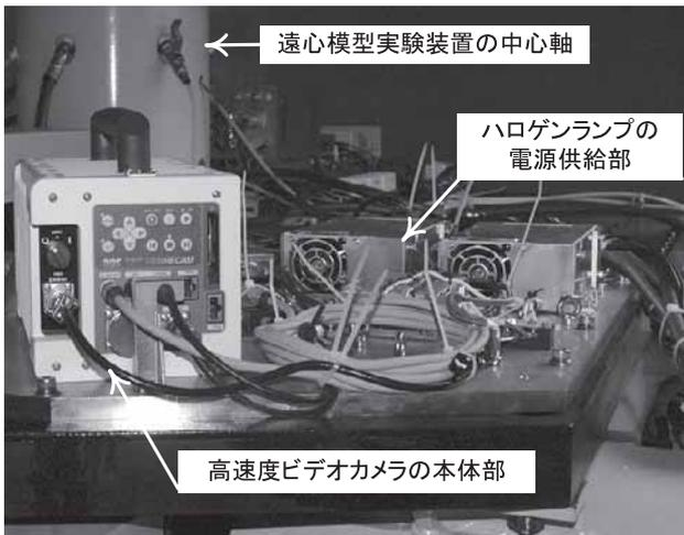
Photo 6 Closed-up view of the high speed camera.
