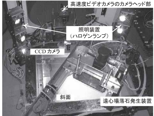
Photo 7 Closed-up view of the camera head and lighting system.
