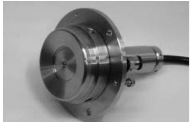
Photo. 2 Air-purge-type electrostatic field sensor.
