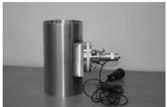
Photo. 3 Electrostatic field detector for pipe.
