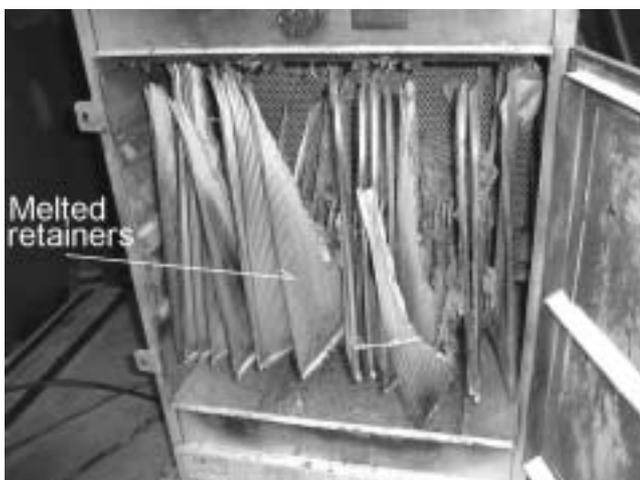
Fig. 1 A dust explosion in a bag-filter device during retrieving collected magnarium dust.
