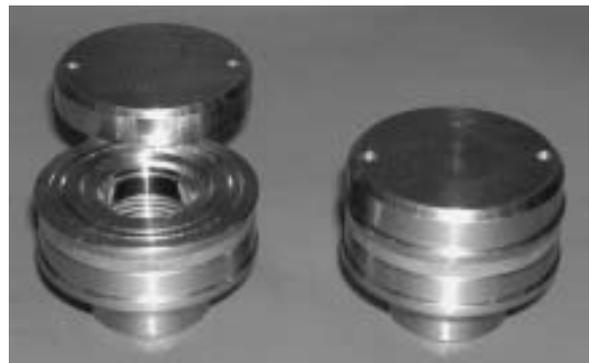
Photo. 3 Improved type of magnetic safety valve.
