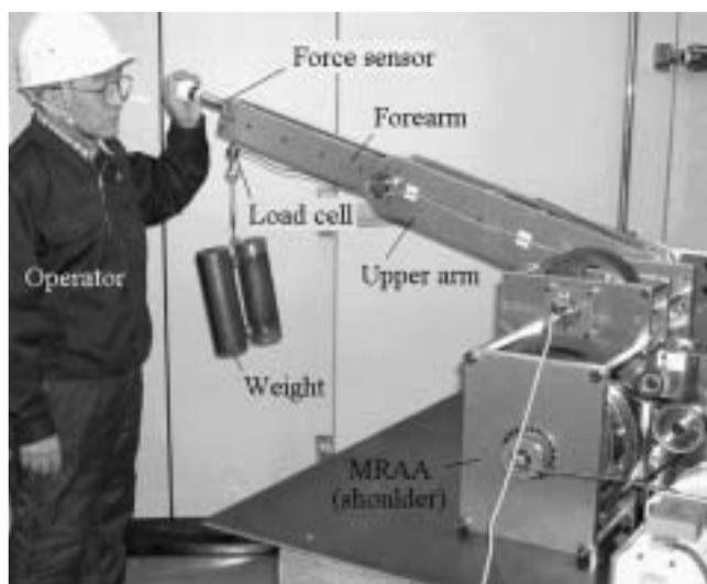
Photo 4 Experiment of cooperative material handling using experimental robot arm.
