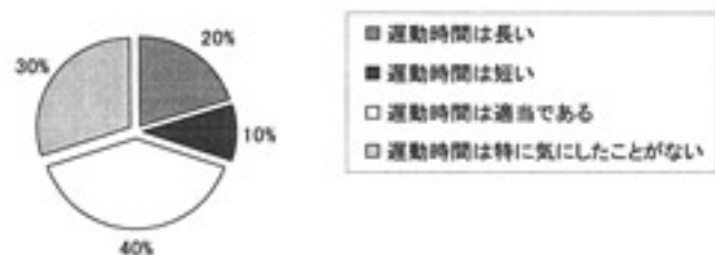
Fig. 35 Degree of usability during the delay time of an AC arc-welding machine with a VRD until it reduces the no-load voltage to safety voltage. (under temporary welding conditions) 仮溶接における運動時間の長さの印象 (テストボタンによる動作)
