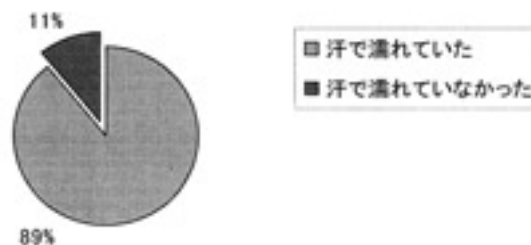
Fig. 19 Influence of wet condition of work clothes on electric shock. 感電時の作業着衣の状況
