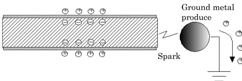
(c) Moving the rod close to ground metal produces a spark discharge.
