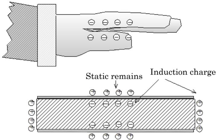
(b) A static charge remains in the coating on the metal rod after the shaft is released (induction charge).
