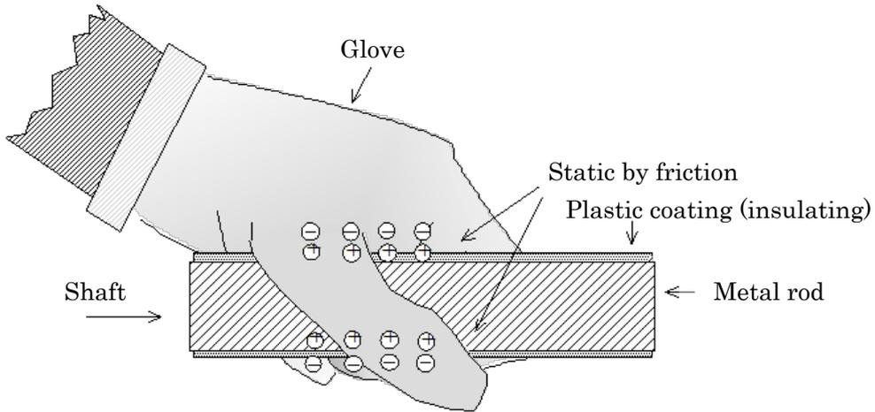
(a) Friction between glove and plastic coating causes static.
