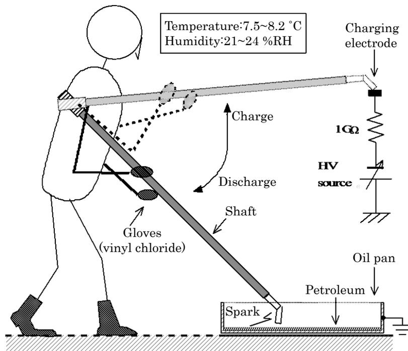
Figure 6. Ignition test of petroleum with charged scraper
