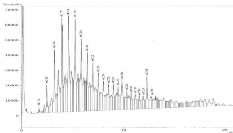
(b) Composition of non-volatile components of the sludge (petroleum wax)
