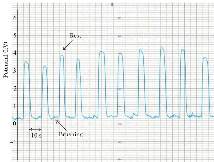
Figure 7. Potential change of the scraper during scraping
