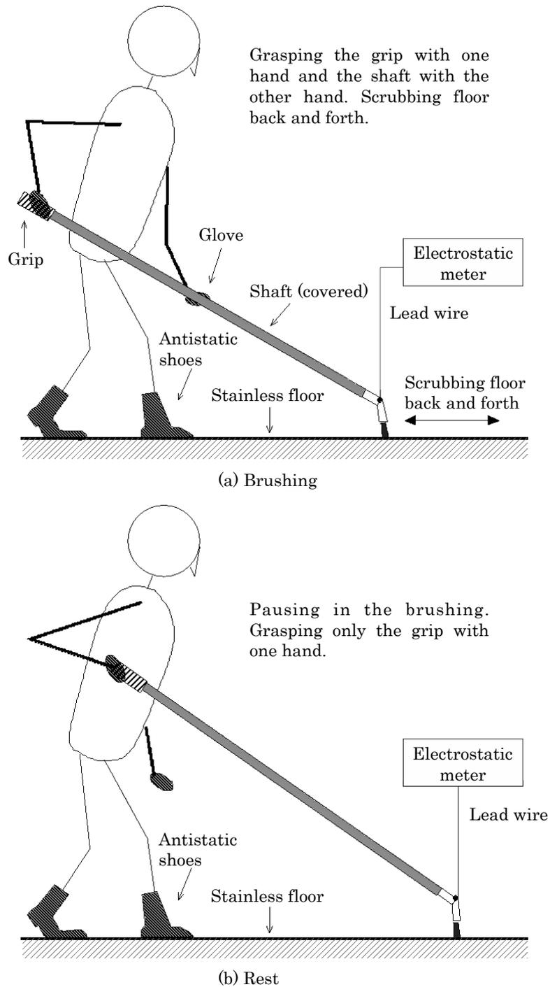
**Figure 5. Experiment to determine static electricity generated during scraping**
