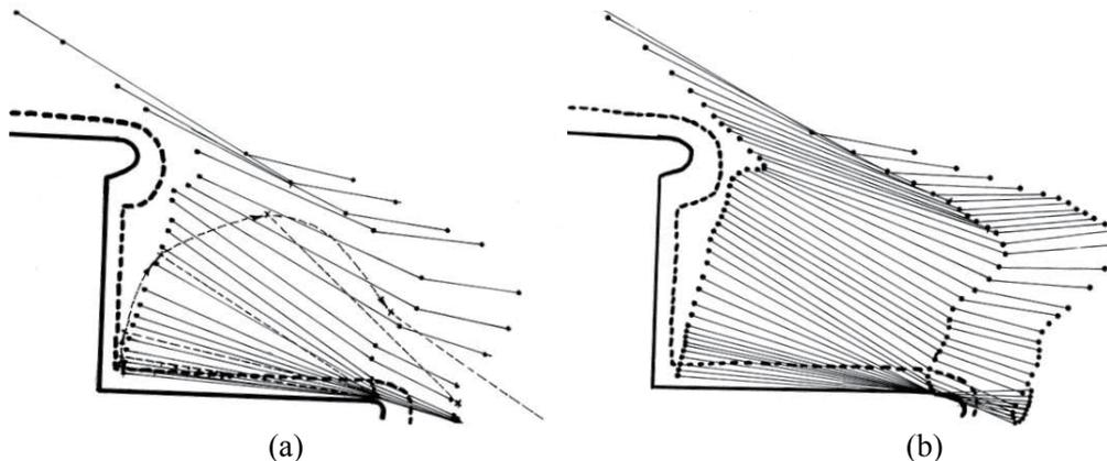
**Figure 5. Analyses, from video, of two descents of a mocked up home stair, both showing interactions of step geometry and descent gait of one shod foot, with back of shoe heel, ball of the foot and front of the shoe sole indicated in two-segment lines each 1/24 second apart**
