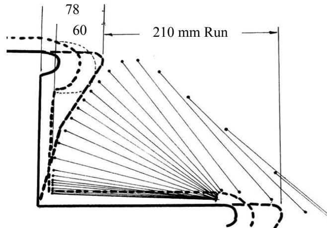
**Figure 6. Analysis of foot pivot on lift off from a home stair tread as a basis for a redesign of the interface of the nosing and closed riser, preferably with a compound back slope**
