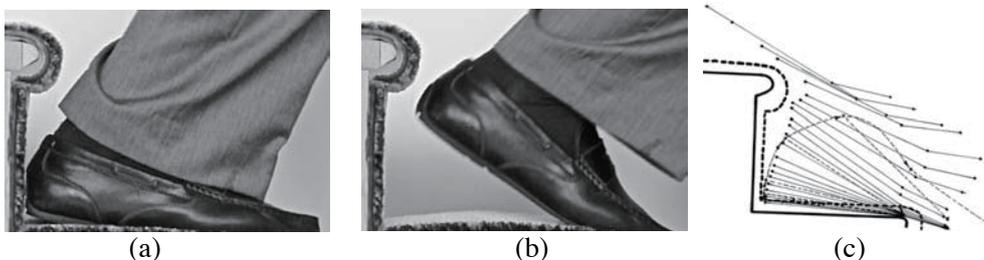
**Figure 1. Lift off portion of descent down home stair mock up shown photographically in (a) and (b) with frame-by-frame analysis of complete use of this step shown in (c)**
