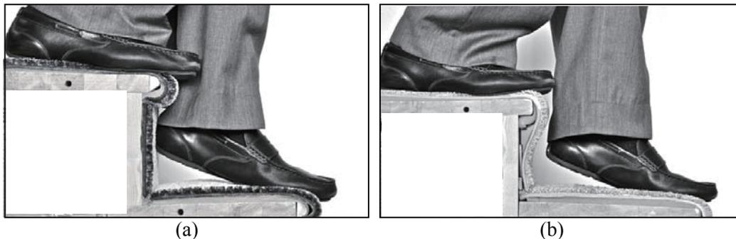
**Figure 2. Mockups of (a) typical Canadian home stair and (b) typical public stair, both carpeted but with different carpet treatments that would meet typical code requirements prohibiting abrupt lips of projecting nosings, but only on public stairs**
