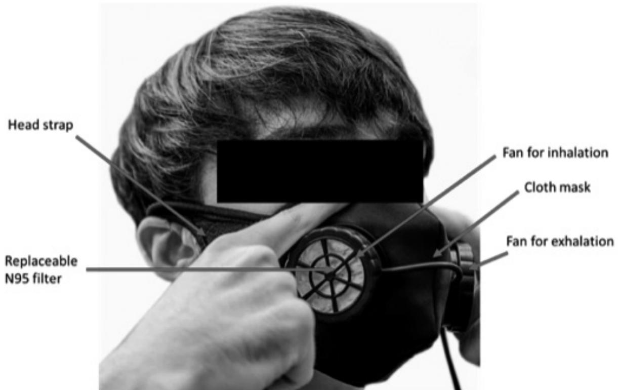
Fig. 2. Components of PAPR (2 fans, N95 filter).
