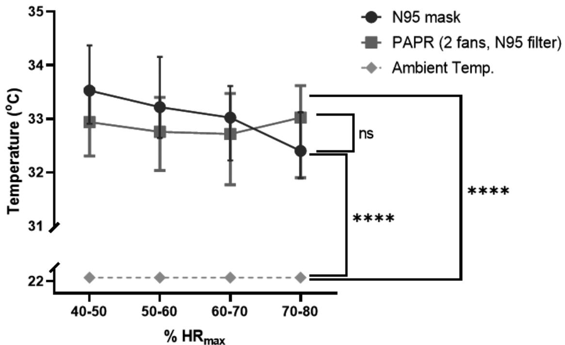
Fig. 6. Changes in temperature inside the N95 mask and PAPR (2 fans, N95 filter) during incremental exercise. (%HR<sub>max</sub>, percentage of maximum achievable heart rate, \*\*\*\* represents  $p$ -value < 0.0001, ns not significant)
