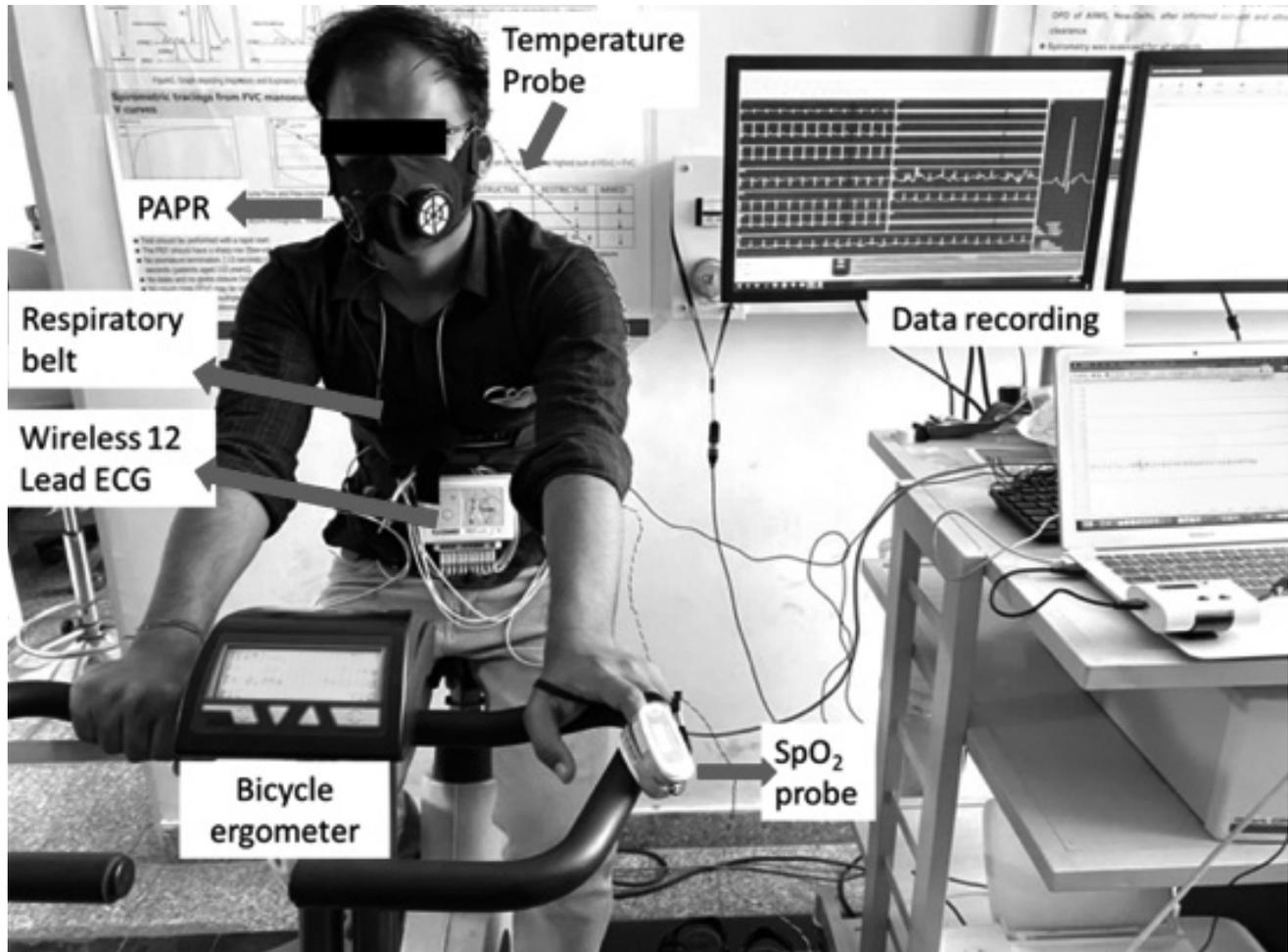
**Fig. 1.** Recording setup showing the subject performing incremental exercise protocol, wearing PAPR (2 fans and N95 filter). ECG, respiration, SpO<sub>2</sub>, and temperature were continuously recorded.
