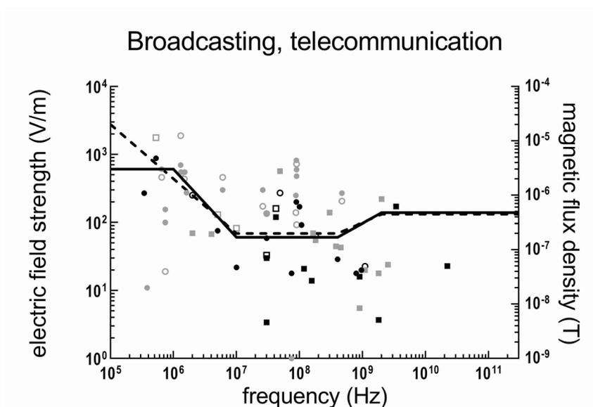
Fig. 4. Maximum electric field strength (left y-axis) and magnetic flux density (right y-axis) at the worker's position per publication, per main frequency component for broadcasting and telecommunication antennas.
