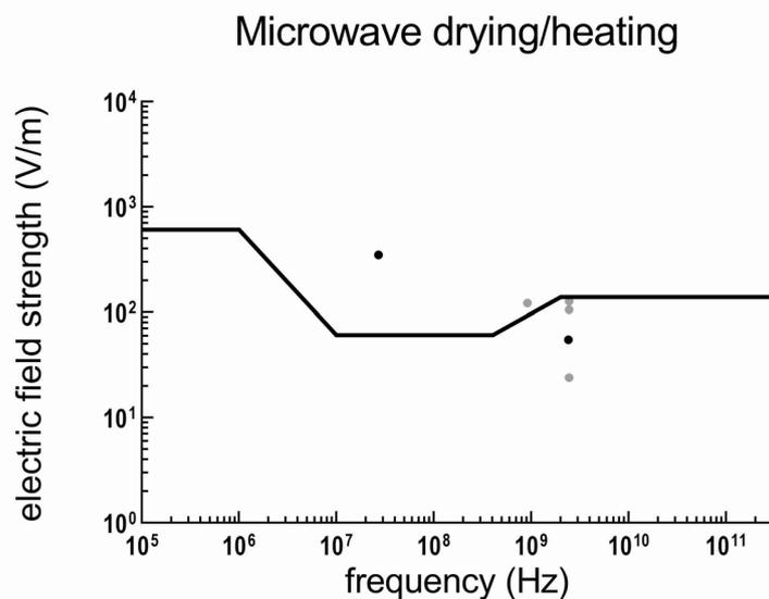
Fig. 5. Maximum electric field strength at the worker's position per publication, per main frequency component for industrial drying or heating processes.
