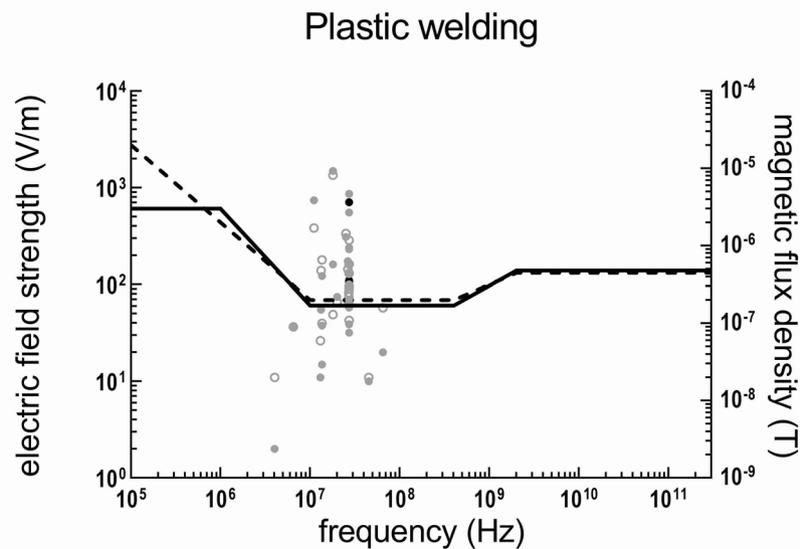
Fig. 1. Maximum electric field strength (left y-axis) and magnetic flux density (right y-axis) at the worker's position per publication, per main frequency component for dielectric heating of plastic.
