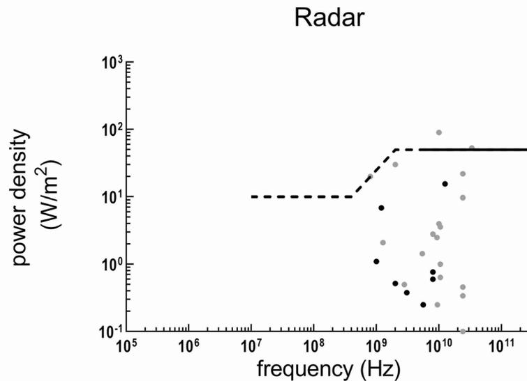
**Fig. 6.** Maximum equivalent plain wave power density at the worker's position per publication, per main frequency component for radar devices.
