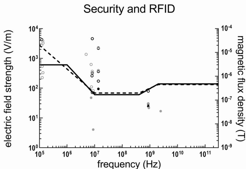
**Fig. 2.** Maximum electric field strength (left y-axis) and magnetic flux density (right y-axis) at the worker's position per publication, per main frequency component for security gates and scanners and RFID transmitters or active transponders.
