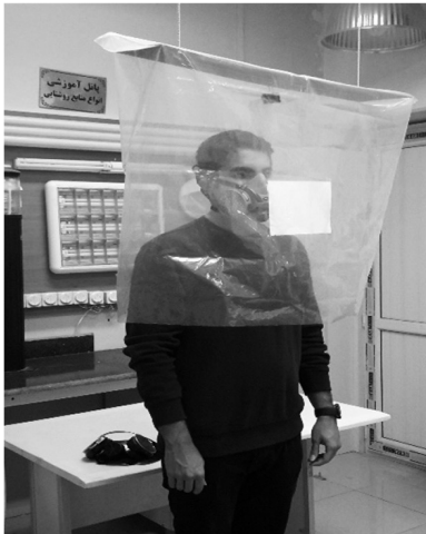
Fig. 1. The participant was inside the test hood during the IAA fit testing procedure.
