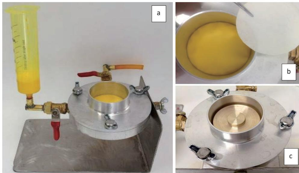
**Fig. 1.** (a) Left: Side view of cell 1 mounted on a stand. (b) Right top: Collector disc being placed on top of the elastomeric material (yellow chemical in the chamber below the sample is visible through the translucent material). (c) Right bottom: Weight placed on top of the collector disc to ensure contact with material.
