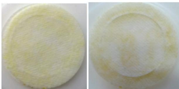
Fig. 8. High variability in a permeation observed in collector discs placed below material with microporous surface and spunbond backing.
