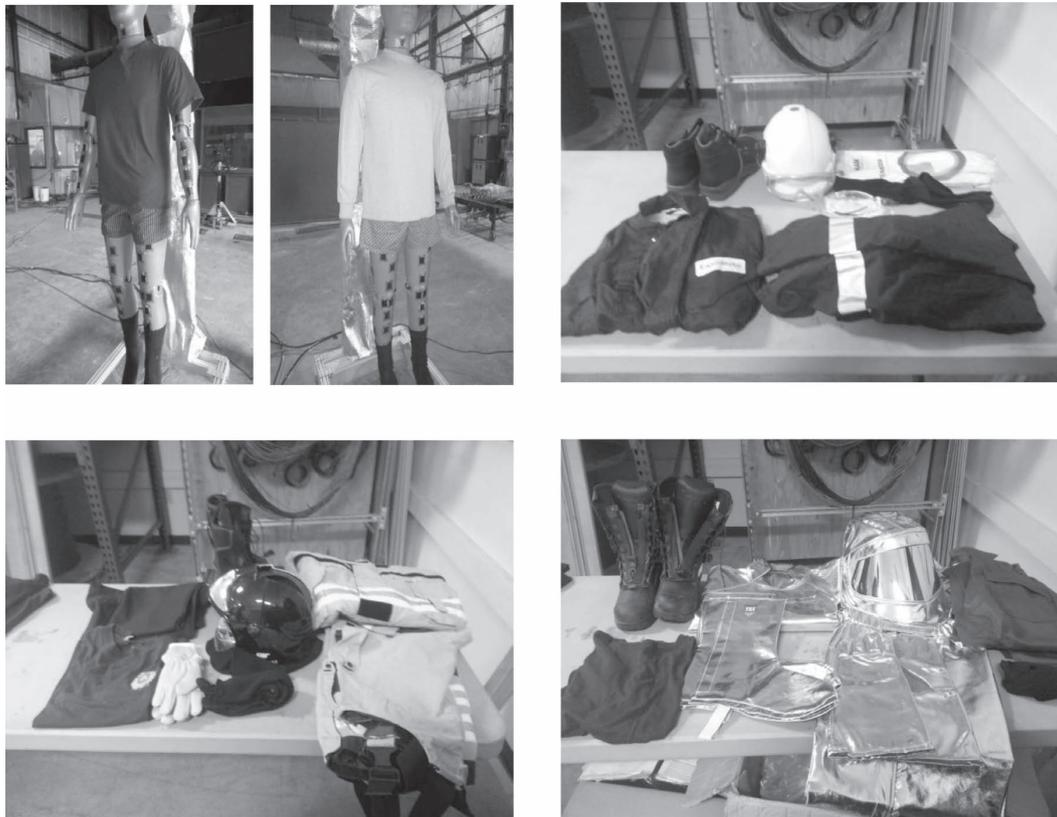
**Fig. 1. Clothing ensembles; upper left under garments, upper middle long sleeve undershirt<sup>\*)</sup>, upper right operator's clothing, lower left firefighter's clothing, lower right aluminized clothing.**
