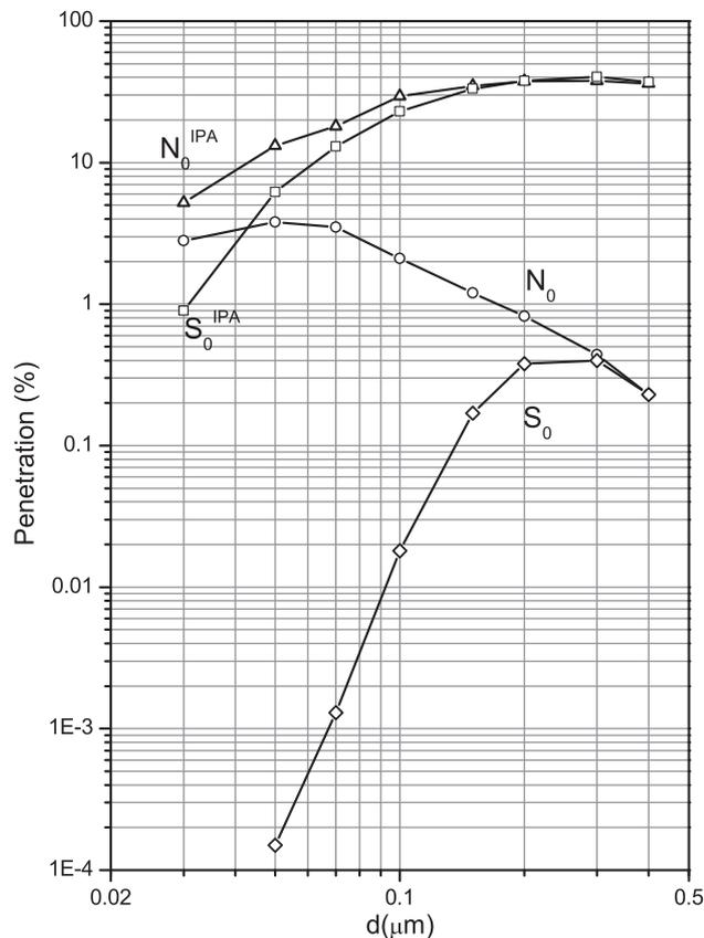
Fig. 2. Neutralized and singly charged DEHS aerosol penetration curves at 0 mg of oil paraffin load (unloaded case) through an untreated ( $N_0$ ,  $S_0$ ) and through an IPA-treated ( $N_0^{IPA}$ ,  $S_0^{IPA}$ ) facepiece.
