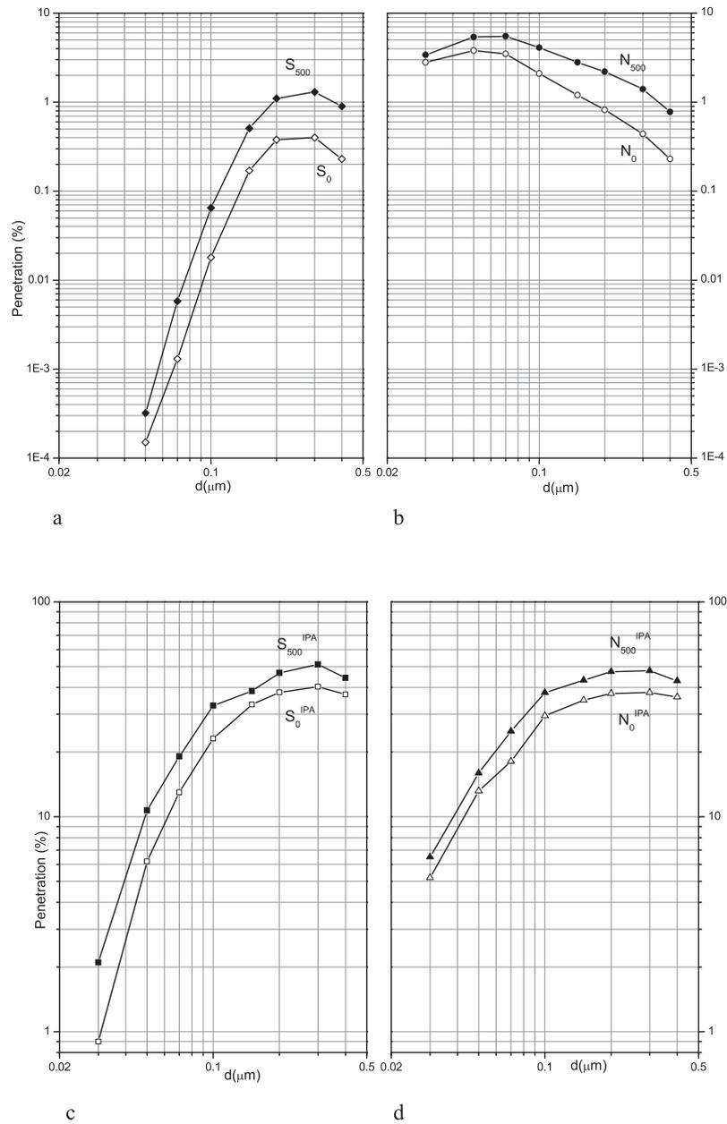
**Fig. 3.** Comparison between penetration curves at 0 mg and 500 mg of paraffin oil load through an untreated facepiece with singly charged (a) and neutralized aerosol (b) and through an IPA treated facepiece with singly charged (c) and neutralized aerosol (d).
