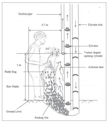
b. Incorporation of cylinder at feeding section
