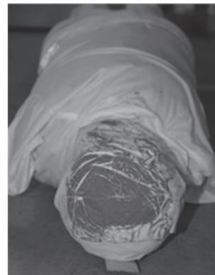
Fig. 7. Damage observed on the parietal area of the dummy in the case of impact on the tread.
