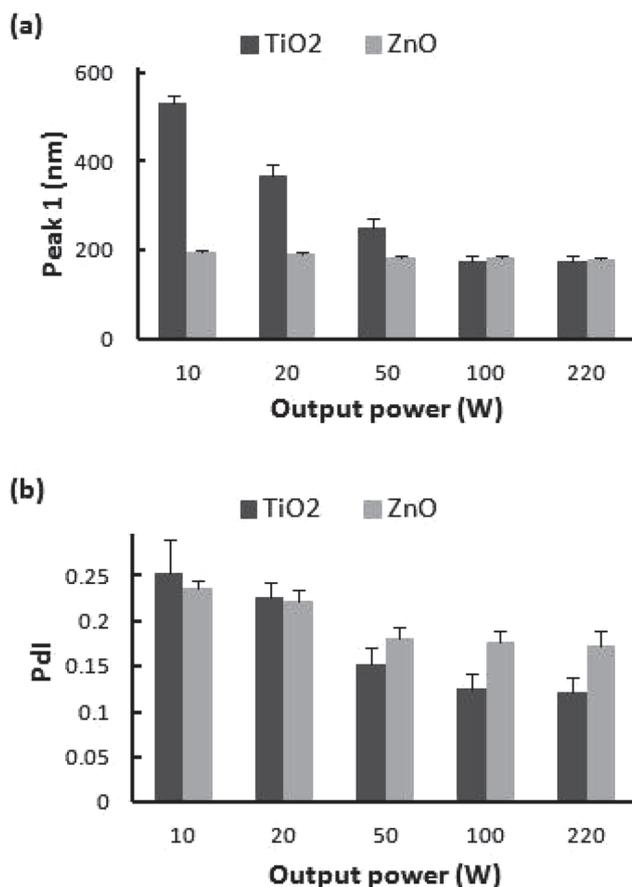
**Fig. 7.** Size characterization of TiO<sub>2</sub> and ZnO nanoparticle suspensions at concentration of 0.5 mg/ml dispersed by a cup-type sonicator at 10, 20, 50, 100, or 220 W, 80% pulse mode, for 10 min: (a) peak 1 and (b) Pdl. Data are mean  $\pm$  SD.
