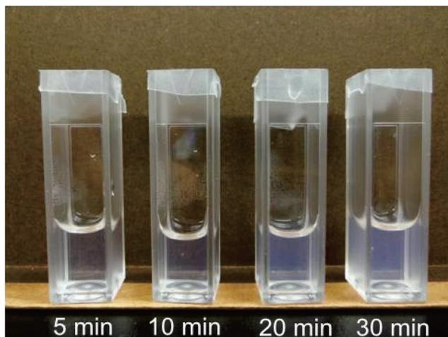
**Fig. 5.** Change in the turbidity of filtered TiO<sub>2</sub> nanoparticle suspensions dispersed by a probe-type sonicator at 20 W, 80% pulse mode, for 5, 10, 20, or 30 min at concentration of 0.5 mg/ml.
