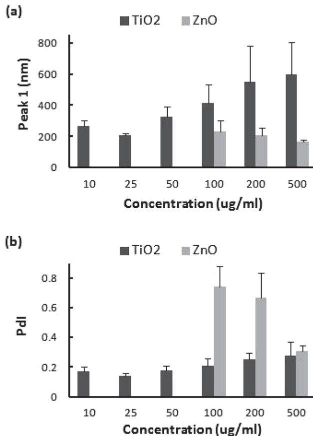
Fig. 1. Size characterization of TiO<sub>2</sub> and ZnO nanoparticle suspensions at concentration of 0.5 mg/ml dispersed by a probe-type sonicator at 20 W, 80% pulse mode, for 30 min, being measured by DLS at concentrations of 10, 25, 50, 100, 200, and 500  $\mu\text{g/ml}$ : (a) peak 1 and (b) PDI. Data are mean  $\pm$  SD.
