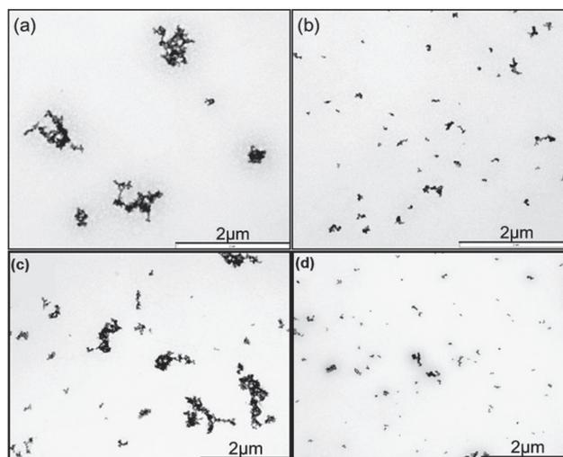
Fig. 4. TEM micrographs of TiO<sub>2</sub> nanoparticle suspensions at concentration of 0.5 mg/ml dispersed by (A) a probe-type sonicator at 20 W, 80% pulse mode, for (a) 10 min and (b) 30 min; (B) a cup-type sonicator at (c) 50 W and (d) 100W, 80% pulse mode, for 10 min.
