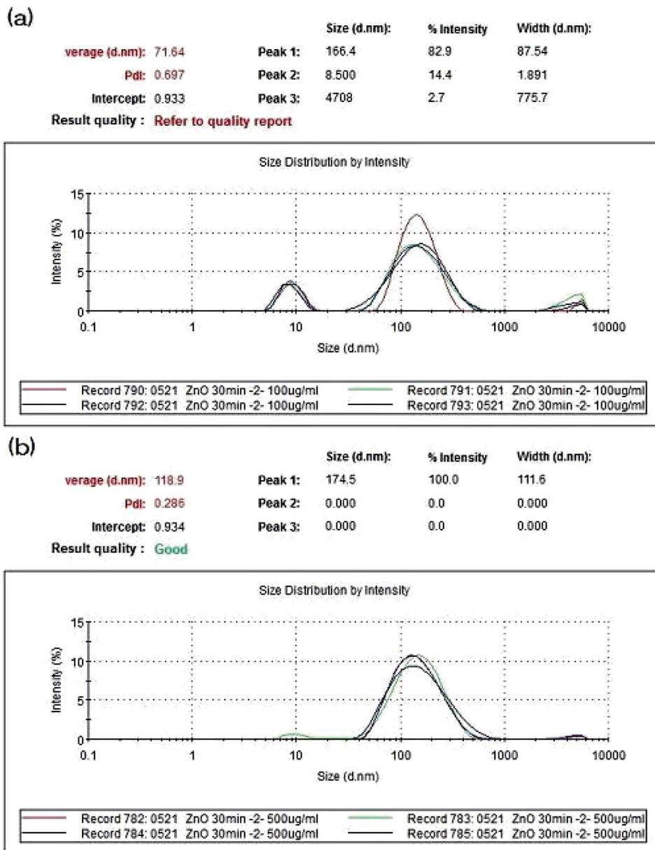
Fig. 2. Report of size distribution of ZnO nanoparticles suspensions dispersed by a probe-type sonicator at 20 W, 80% pulse mode, for 30 min, at measure concentrations of: (a) 100 and (b) 500  $\mu\text{g/ml}$ .
