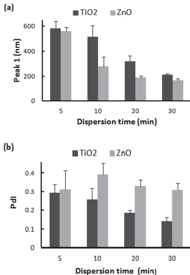
Fig. 3. Size characterization of TiO<sub>2</sub> and ZnO nanoparticle suspensions at concentration of 0.5 mg/ml dispersed by a probe-type sonicator at 20 W, 80% pulse mode for 5, 10, 20, or 30 min: (a) peak 1 and (b) PDI. Data are mean  $\pm$  SD.
