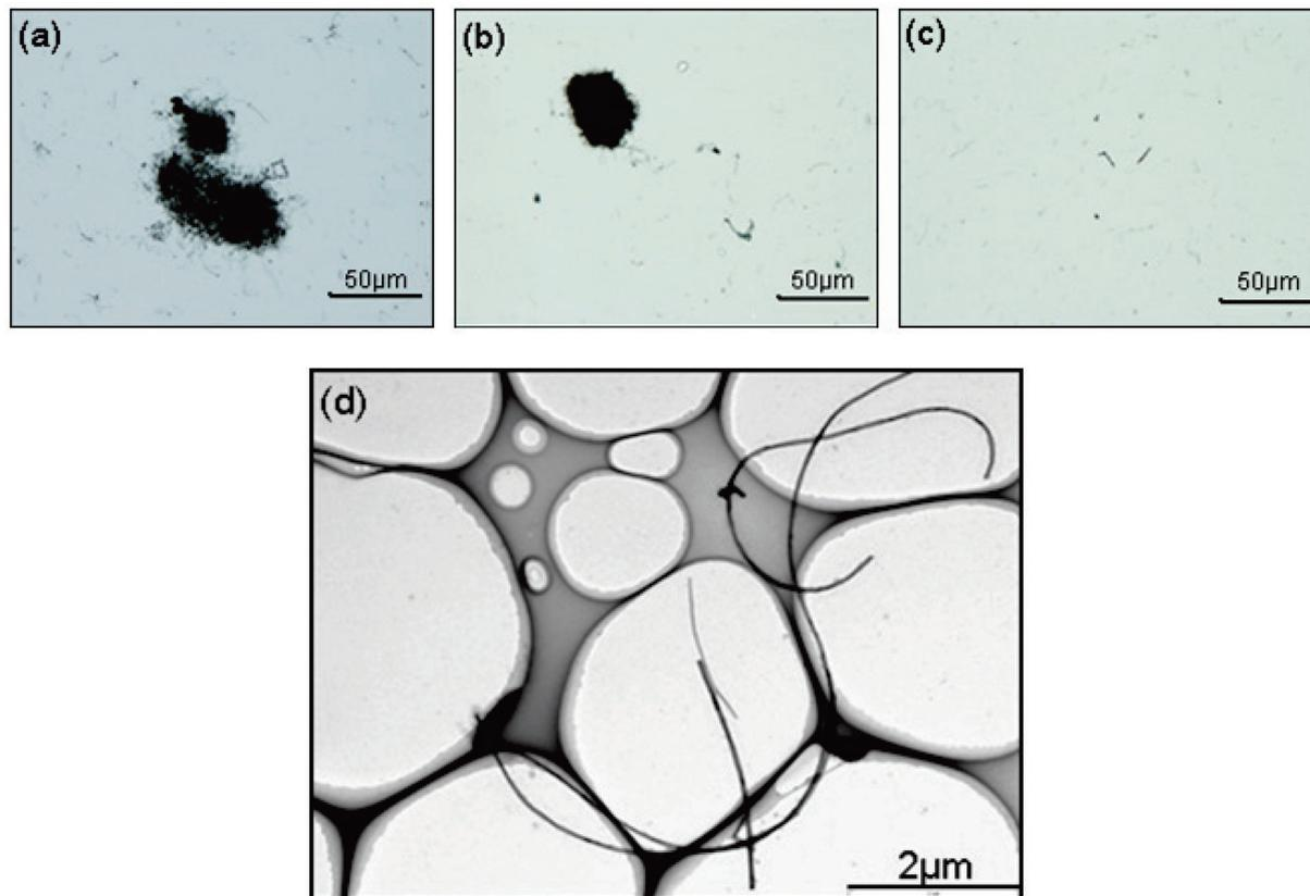
**Fig. 8.** Optical microscope micrographs of MWCNT suspensions at concentration of 2.0 mg/ml: (a) un-dispersed, (b) dispersed by a cup-type sonicator at 100 W, 80% pulse mode, for 10 min, and (c) for another 10 min; and (d) TEM micrograph of MWCNT sonicated twice.
