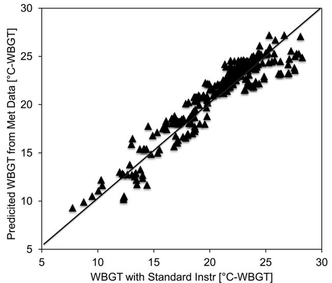
Fig. 1. Comparison of WBGTs from the standard instrument cluster to the predicted from meteorological data using Equation 1. The identity line is shown.
