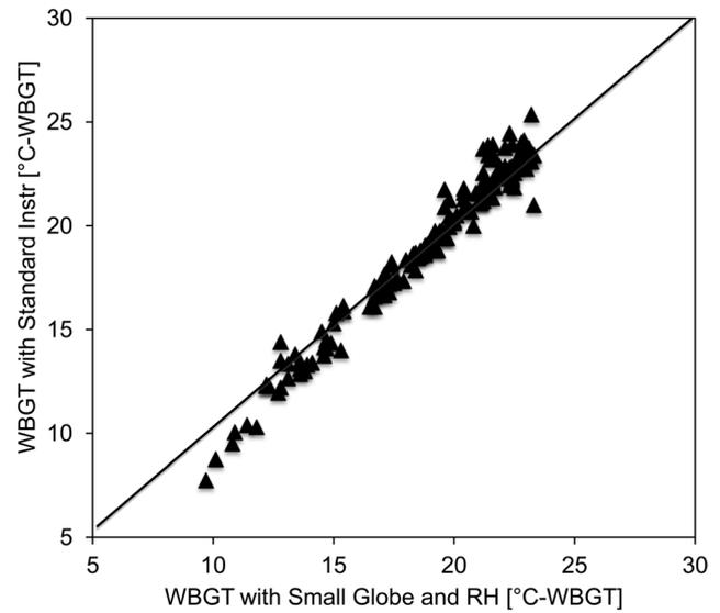
**Fig. 3.** Comparison of WBGTs from the standard instrument cluster to the electronic device with a small globe and relative humidity sensor.
