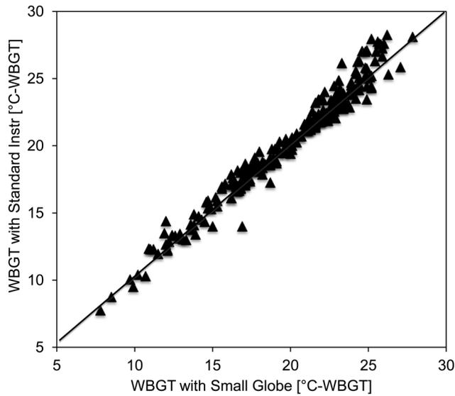
**Fig. 2.** Comparison of WBGTs from the standard instrument cluster to the electronic device with a small globe.
