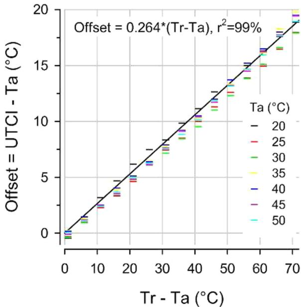
**Fig. 2.** The Offset (=UTCI-Ta) related to the intensity of heat radiation (Tr-Ta) for different values of Ta. The linear regression line with equation and proportion of variance explained (r<sup>2</sup>) are inserted. Wind speed and humidity were set according to the UTCI reference condition.
