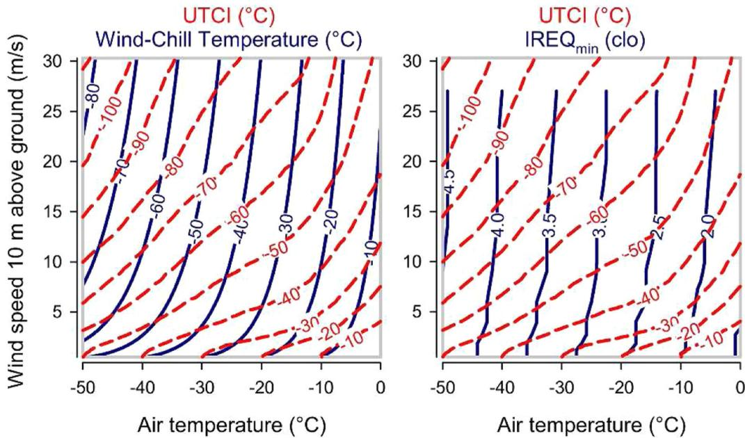
Fig. 6. Contours of UTCI (dashed lines) compared to indices from ISO 11079 (2007), Wind-Chill Temperature (left panel) and minimum Required Insulation (IREQ<sub>min</sub>, right panel) for air temperatures between 0 and -50°C and for wind speeds between 0.5 and 30 m/s. Humidity and radiation were set according to the UTCI reference condition.
