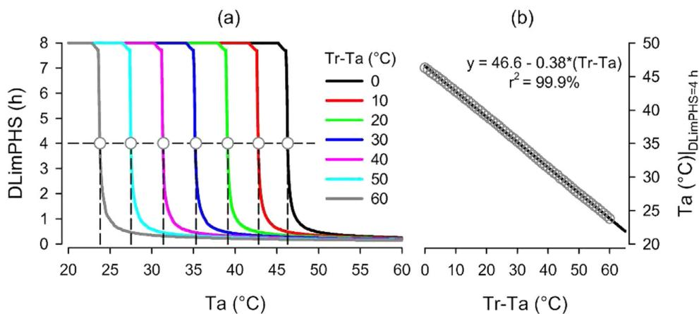
**Fig. 3.** Maximum allowable exposure times (DLim PHS) calculated by PHS related to air temperature for different radiation intensities (a) with circles and dashed lines denoting the half-effective Ta (i.e. Ta with half-maximum DLim PHS = 4 h), whose dependency on radiation intensity expressed by Tr-Ta is depicted in (b).
