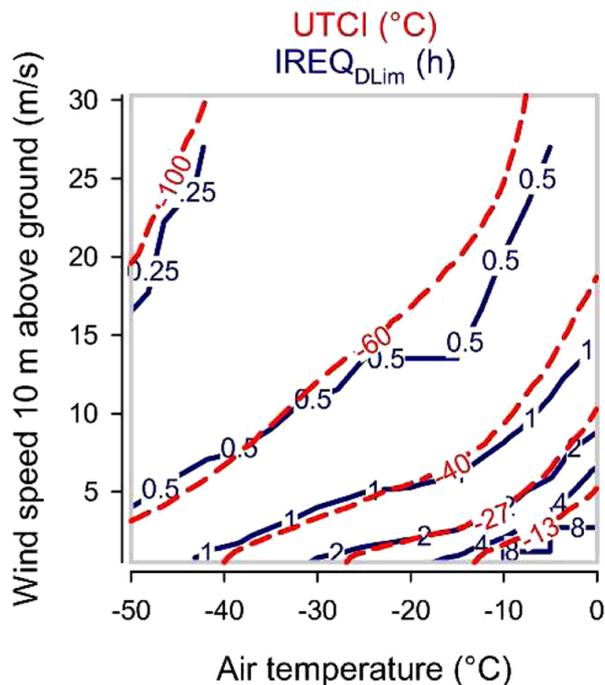
Fig. 7. Contours of UTCI (dashed lines) compared to duration limited exposure (IREQ<sub>DLim</sub>) from ISO 11079 (2007). For environmental conditions cf. Fig. 6. Clothing insulation decreased with air temperature according to the UTCI-clothing model.
