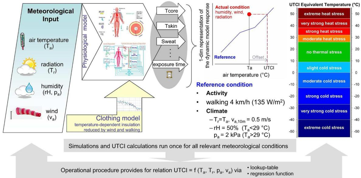
Fig. 1. Elements of the operational procedure and concept of UTCI as categorized equivalent temperature derived from the dynamic response of a thermo-physiological model coupled with a behavioral clothing model.
