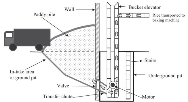
Fig. 1. Drawing of loading area and underground pit in rice mills
