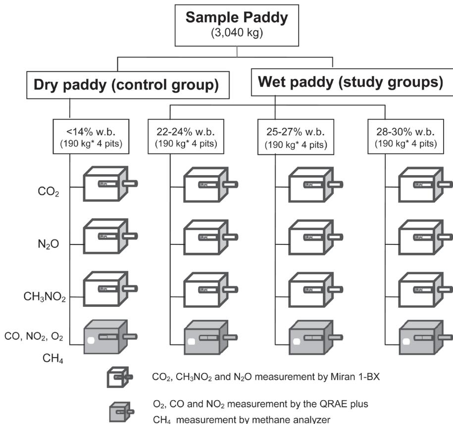
Fig. 3. Schematic of study samples in experimental pits and gas measurement
