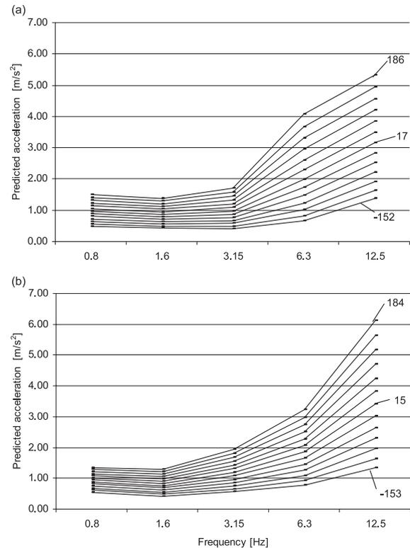
**Fig. 8.** Equivalent intensity contours for arbitrary sensation units from minimum to maximum of the range of value in order to meet the range of definition (range of actually exposed vibration magnitudes) in steps of 12 equidistant units determined from Eq. (14) and Table 5: (a) random octave band-width white noise excitation in x-axis, (b) random octave band-width white noise excitation in y-axis.
