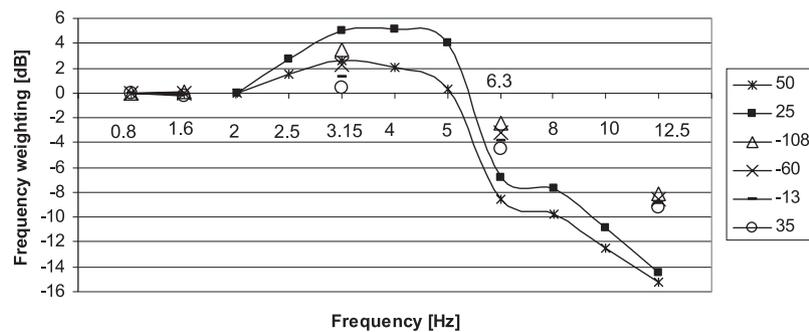
**Fig. 11.** Frequency weightings for vibration exposure in x-direction depending on arbitrary sensation units derived by Morioka (arbitrary units 25 and 50) and in the present study (arbitrary units -108, -60, -13 and 35).
