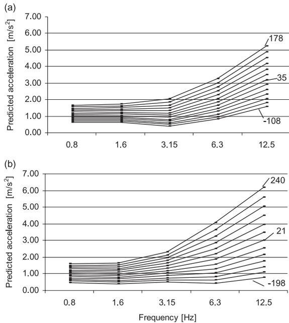
**Fig. 7.** Equivalent intensity contours for arbitrary sensation units from minimum to maximum of the range of value in order to meet the range of definition (range of actually exposed vibration magnitudes) in steps of 12 equidistant units determined from Eq. (14) and Table 5: (a) sinusoidal excitation in x-axis, (b) sinusoidal excitation in y-axis.
