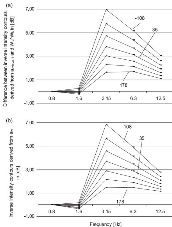
**Fig. 12. (a) Difference between inverse intensity contours depending on arbitrary sensation units in 6 equidistant steps, derived from modified non-weighted overall vibration total values  $a_{ov(n.w.)}$  (referred to 0.8 Hz) and  $W_d \wedge W_k$  in dB for sinusoidal excitation x-direction (see Fig. 9 (a)) (b) Inverse intensity contours derived from weighted overall vibration total values  $a_{ov}$  (referred to 0.8 Hz) in dB.**
