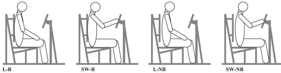
**Fig. 3. Schematic of the postures assumed by test subjects in this study. (L–Hands in Lap; SW–Hands on Steering Wheel; B, NB–with and without Back contact, respectively).**
