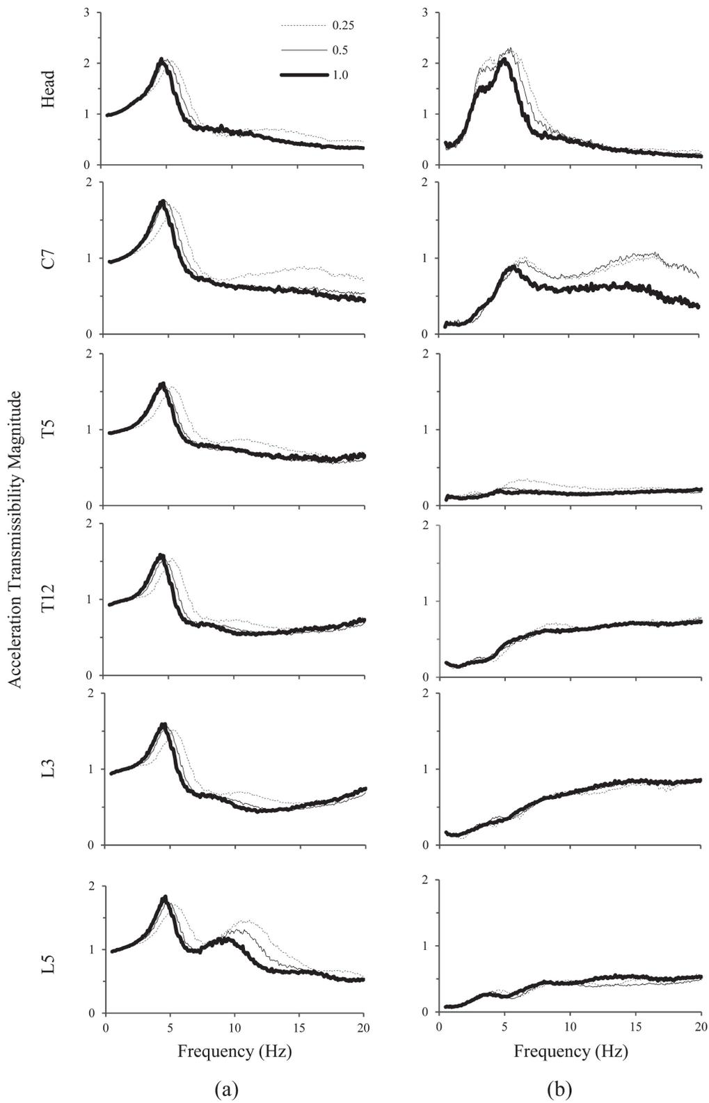
Fig. 8. Influence of vertical vibration on the (a) vertical and (b) horizontal responses of body segments corresponding to the L-NB posture. (Note: Excitation magnitude in the legend is  $\text{m/s}^2$ ).
