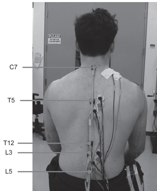
**Fig. 1.** A test subject prior to vibration exposure, instrumented with skin-accelerometers at the indicated vertebral levels (Note: The head strap was secured after the subject mounted the vibration platform for safety reasons).
