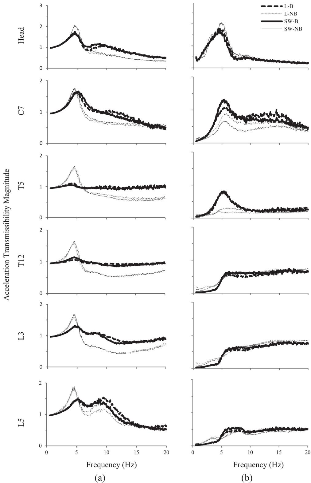
**Fig. 7.** Comparisons of mean responses of the body segments with different support conditions under  $1 \text{ m/s}^2$  vertical excitation. (L-B: Back supported with hands in lap; SW-B: Back supported with hands on steering wheel (SW); L-NB: Hands in lap and no back support; SW-NB: Hands on SW): (a) vertical and (b) horizontal transmissibility magnitude.
