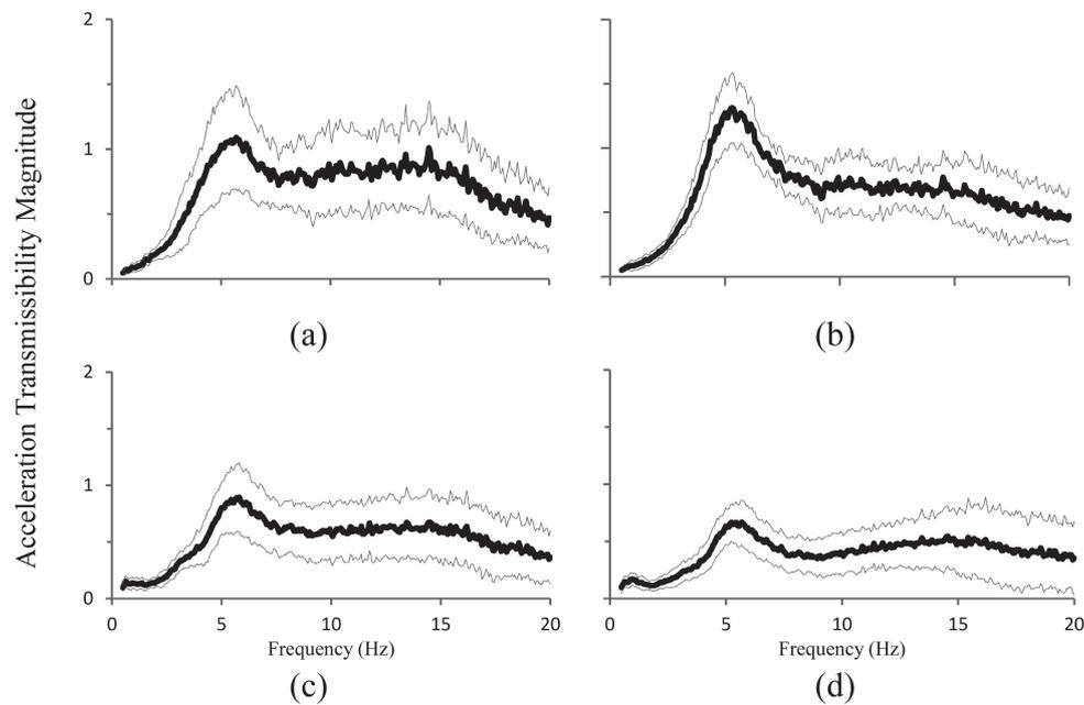
**Fig. 9.** Mean and standard deviation errors of horizontal responses at C7 in the four sitting postures exposed to  $1 \text{ m/s}^2$  seat excitation: (a) L-B; (b) SW-B; (c) L-NB; and (d) SW-NB.
