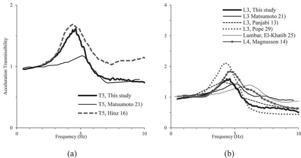
**Fig. 10.** Comparison of mean measured vertical responses at T5 and L3 with the reported data on vibration transmitted to the spine in the (a) thoracic, T5; and (b) lumbar region, L3 and L4.
