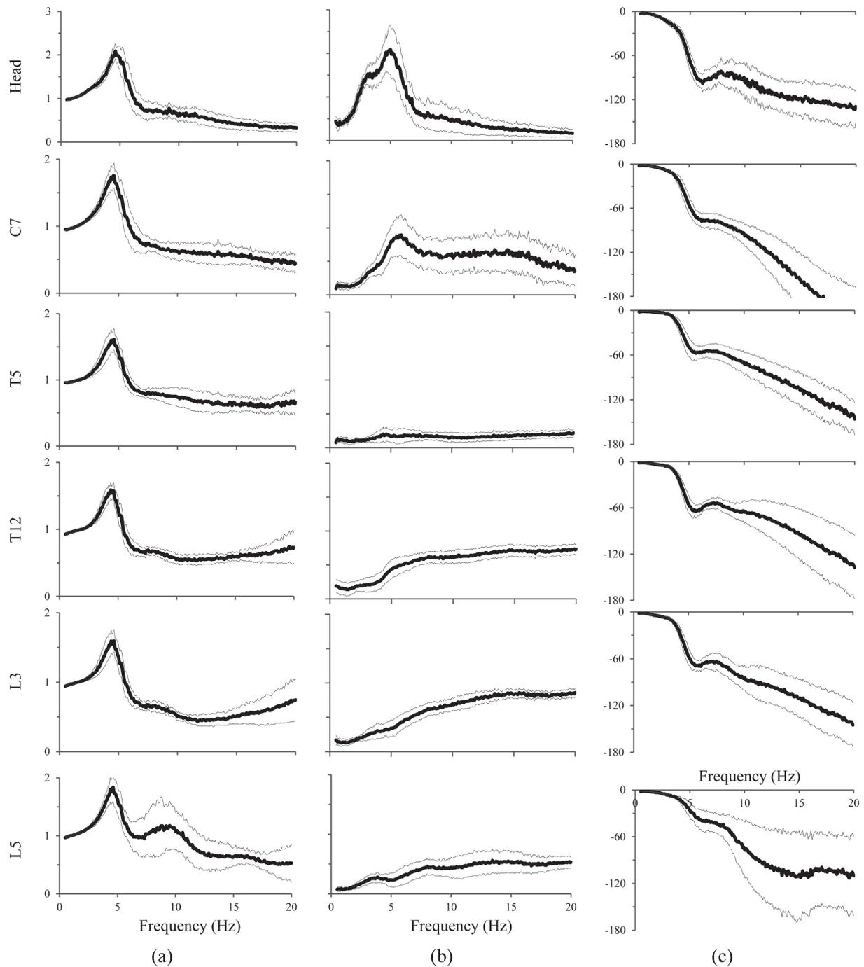
**Fig. 6.** Mean and standard deviation of the mean responses at the measured locations for 12 subjects seated in the L-NB posture and exposed to  $1 \text{ m/s}^2$  vertical excitation: (a) vertical; and (b) horizontal transmissibility magnitude; (c) vertical transmissibility phase (degrees).
