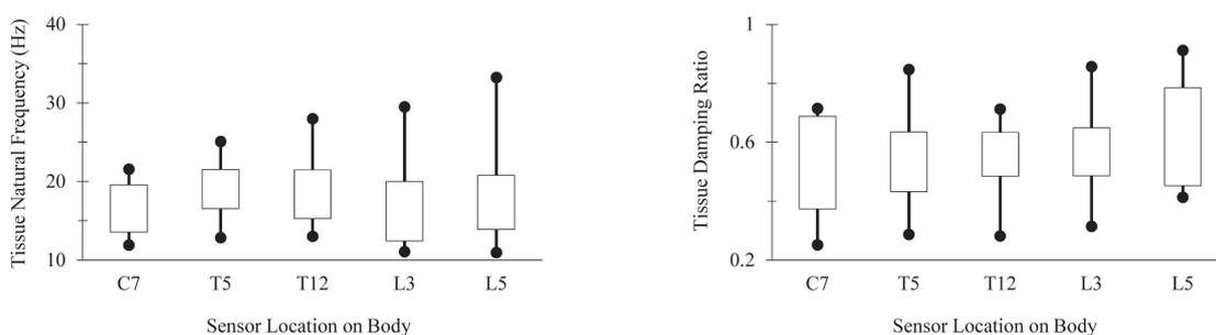
**Fig. 4. Ranges for the values of skin-tissue natural frequency and damping ratio calculated for 12 test subjects through free-vibration (pull) tests on the skin-mounted accelerometers at the measurement locations.**
