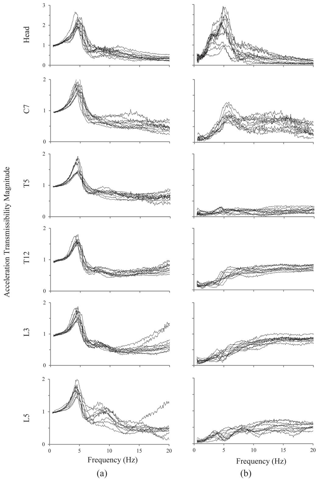
Fig. 5. (a) Vertical and (b) horizontal transmissibility magnitudes measured at different locations of 12 subjects seated in the L-NB posture and exposed to  $1 \text{ m/s}^2$  (RMS) random vertical vibration.
