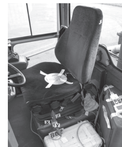
Fig. 1. Whole-body vibration measuring equipment consisting of accelerometers for seat surface and seat mounting point.
