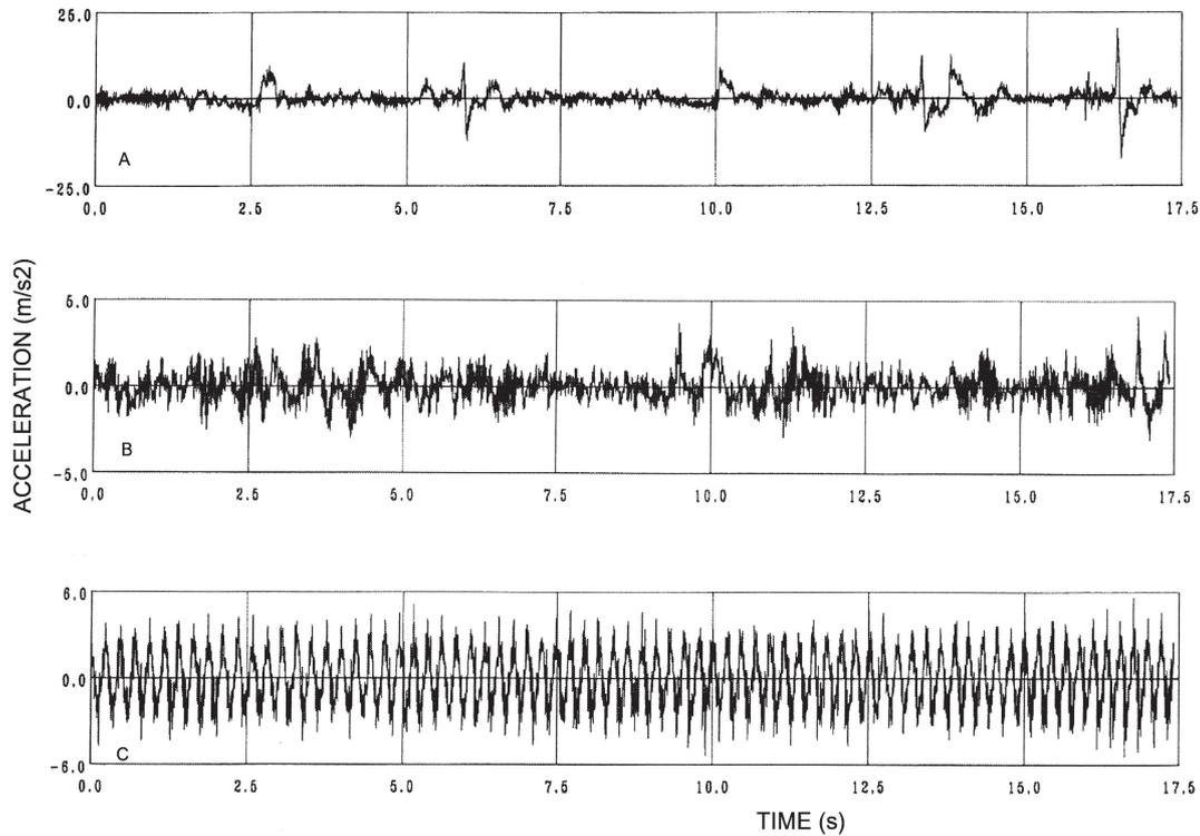
**Fig. 5.** Frequency-weighted acceleration-time history of the Z-direction motion at the seat of a M2HS Bradley fighting vehicle travelling: A - cross country at 20 m.p.h.; B - cross country at 15 m.p.h., and; C - over 6" pitch washboard.
