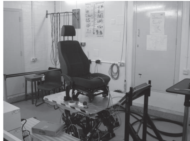
Fig. 1. Six-axis hydraulic shaker at Loughborough University used in the study.
