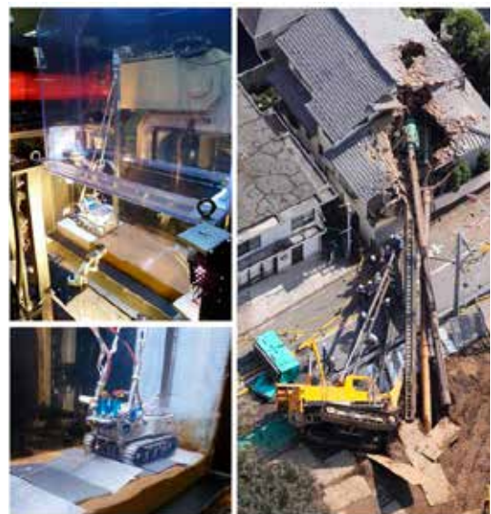
不安定な施工現場を自走するくい打機の転倒危険性に関する研究 The study on potential risk of overturning in drill rigs while self propelling on unstable supporting ground in construction sites.
