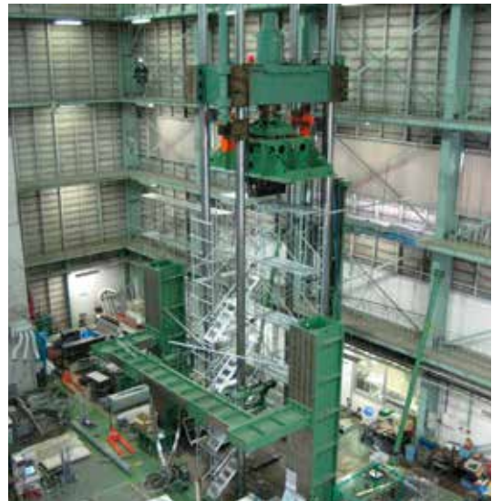
仮設構造物の性能実験 Performance test of temporary structures.
