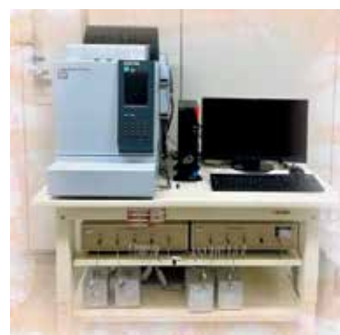
被験物質濃度測定装置 Gas chromatography for Vapor concentration monitor system
