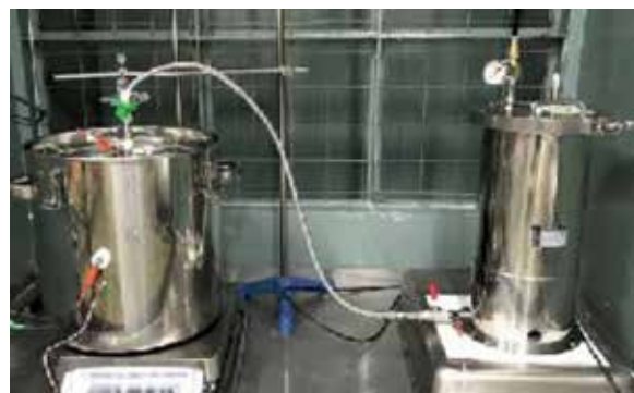
液体の噴霧帯電量の測定 Experimental equipment for measuring of electric charge generated by flow and jet of liquid.
