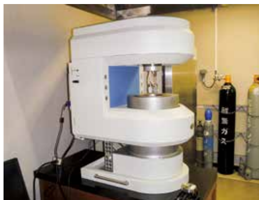
発熱挙動試験用の断熱熱量計 Adiabatic reaction calorimeter for evaluating exothermal behavior.
